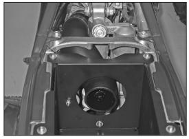
22. Install the K&N® intake tube through the air box into the silicone hose on the carburetor. Secure the intake tube to the mounting bracket on the air box with the hardware provided and to the silicone hose with the provided hose clamp.
