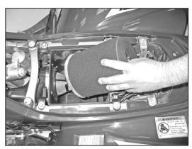
6. Loosen the air filter retaining bolt and then remove the stock air filter from the air box.
