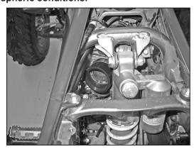
16. Install the silicone hose onto the carburetor and secure with the provided hose clamp.
