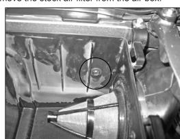
7. Push the crank case vent fitting and grommet out of the air box from the inside out to remove it from the air box.
