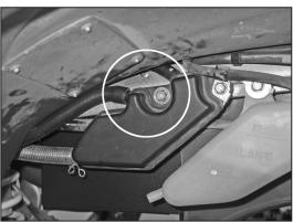
21. Route the crank case breather hose to the vent chamber and then connect it to the open end of the crank case vent port.
