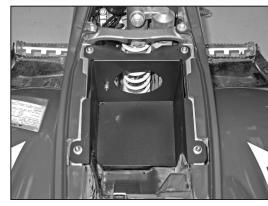
20. Install the air box into the chassis as shown and secure with the provided hardware.
