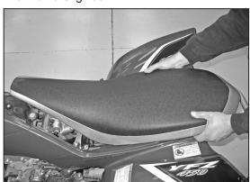
2. Release and remove the seat from the vehicle as shown.
